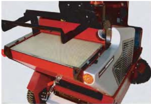
Large High Efficiency Dust Filtration
